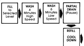
IMPORTANT: THE WASHER WILL PAUSE BRIEFLY THROUGHOUT EACH CYCLE. These pauses are normal. They allow for the reversing of the motor, normal washer operations, and the cool down portion of the PERMANENT PRESS Cycle.
